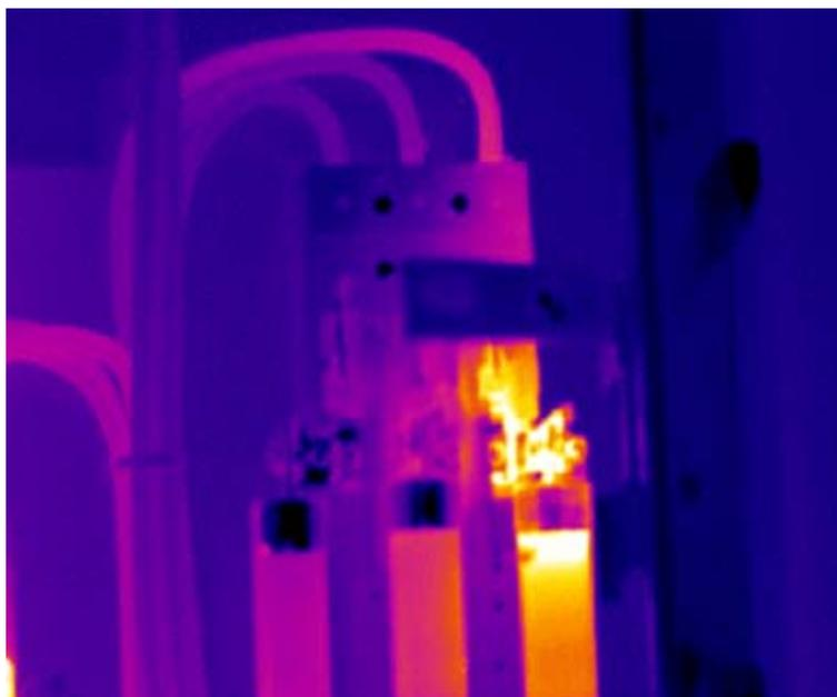
**Fig.15 Inspection of connectors**
