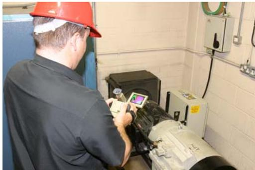
**Fig 2. The inspection of electrical equipment using a Thermal Imager**
